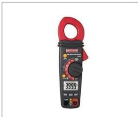
The Clamp Ammeter measures voltage and amperage both on Ac and DC modes. It is used during the Screening and the Branding steps of our battery reconditioning process.
