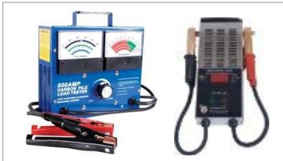
The Carbon Pile Tester (500Ah) is used to test the state of health of all deep cycle batteries of 6, 8, and 12 volts. The 100Ah load tester is used to test cranking batteries during our Screening and Branding step. Our battery recovery training fully teaches how to use this tool.
