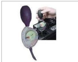
The Hydrometer is used to measure the specific gravity of the electrolyte. This tool is used during our Screening step and during our Branding step of our battery reconditioning process. You will receive three hydrometers.
