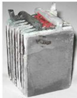
Cell pack with corrosion & sulfation in both plates.
